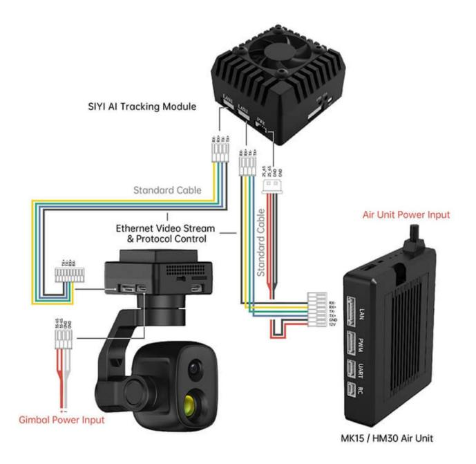
4. Please refer to the picture below to connect SIYI gimbal camera with flight controller and integrate attitude data.
